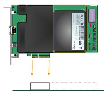
5. Insert the Luna PCI-E card, gently but firmly, into the connector. It should go straight in – angling the card might
