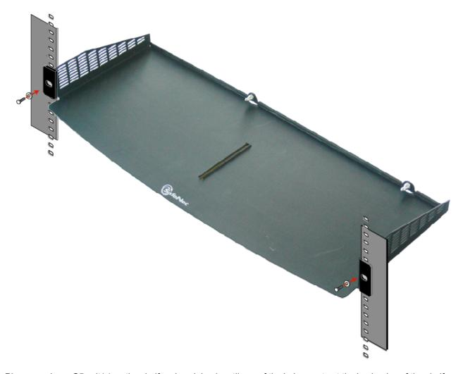
2. Place your Luna G5 unit(s) on the shelf and push back until one of the index posts at the back edge of the shelf engages the index hole on the back panel of each Luna G5.
