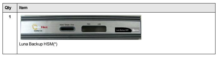
(\* The SafeNet Luna Backup HSM is a backup-storage option, suitable for off-site storage, and for backing up multiple HSM partitions. Its contents are automatically secured at the same level of authentication security (Password versus PED) as the HSM it is backing up. The Luna Backup HSM can be connected directly [locally] to an HSM, or it can be connected to a computer to backup remotely located HSMs, in conjunction with Remote PED.)
